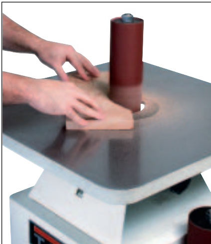
The 38 mm spindle stroke provides a scratch-free finish and prolongs sleeve life
